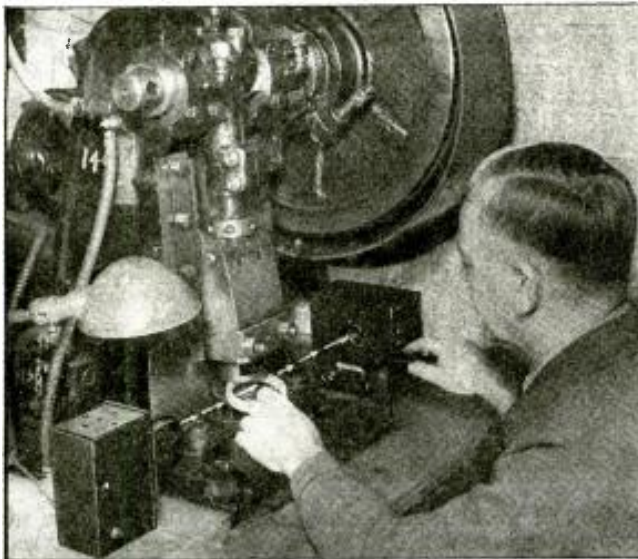
These photos illustrate but 2 of the thousands of industrial applications for photoelectric equipment. The illustration at the left shows photoelectric equipment used to assure the safety of the operator of a heavy punch-press. The illustration at the right shows the same photoelectric equipment, here used to count radio speakers as they pass along on an endless belt.
